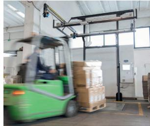
Weight and volume measuring systems for pallets can indeed have several strengths thanks to their different configurations. These allow them to obtain the weight, volume and image of pallets, along with different products and shapes, including certified measure ment of regular and irregular items like tires, fabric rolls and more.
